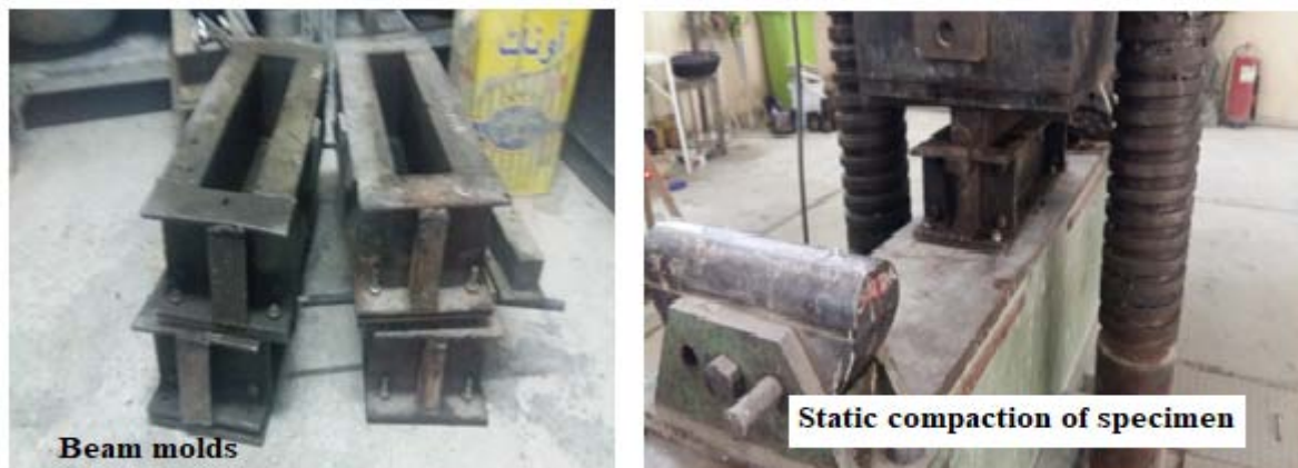
Fig.2. Preparations of Beam specimens
