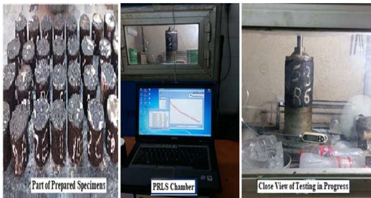
Fig.4. The Repeated Compressive Stress Testing Apparatus
